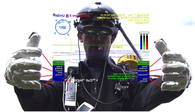
(a) Tinmith glove based input description.
